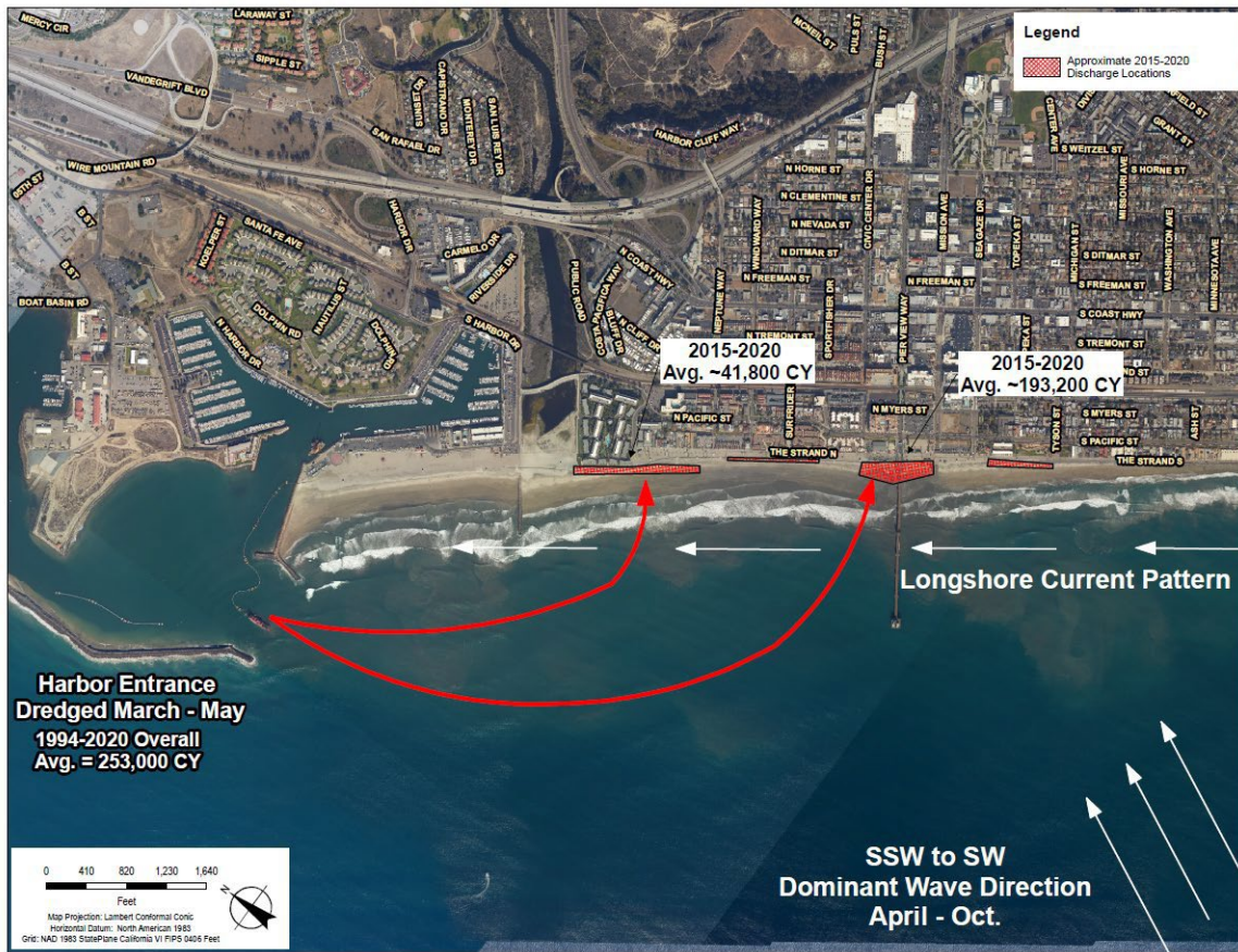
Figure 4-2. USACE Sand Placement Relative to Seasonal Longshore Transport Schematic
