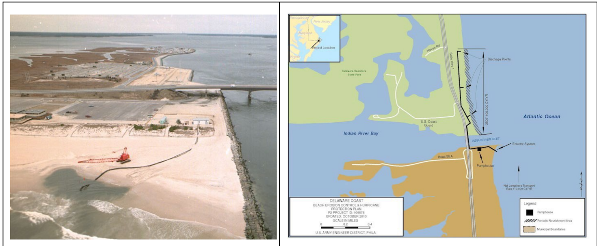
Figure 11-3. Mobile Sand Bypass Option – Indian River Inlet, Delaware (USACE, 2021)
