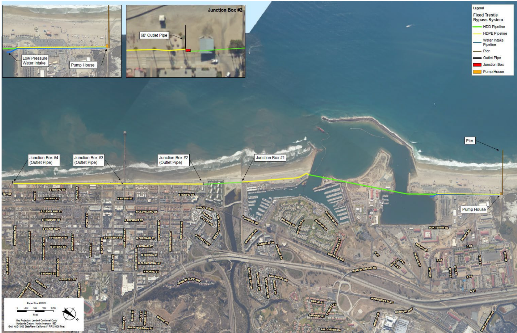
Figure 11-1. Fixed Trestle Sand Bypass Option
