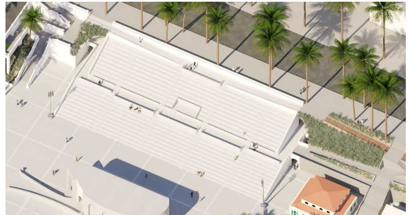
N. PACIFIC STREET LEVEL The sidewalk abutting the amphitheater is widened to a dimension equal to sidewalk width at the Pier Bridge entrance. It is designed to accommodate large crowds entering and exiting the venue. Landscape planting areas descend from N. Pacific Street and follow the profile of the coastal bluff.
