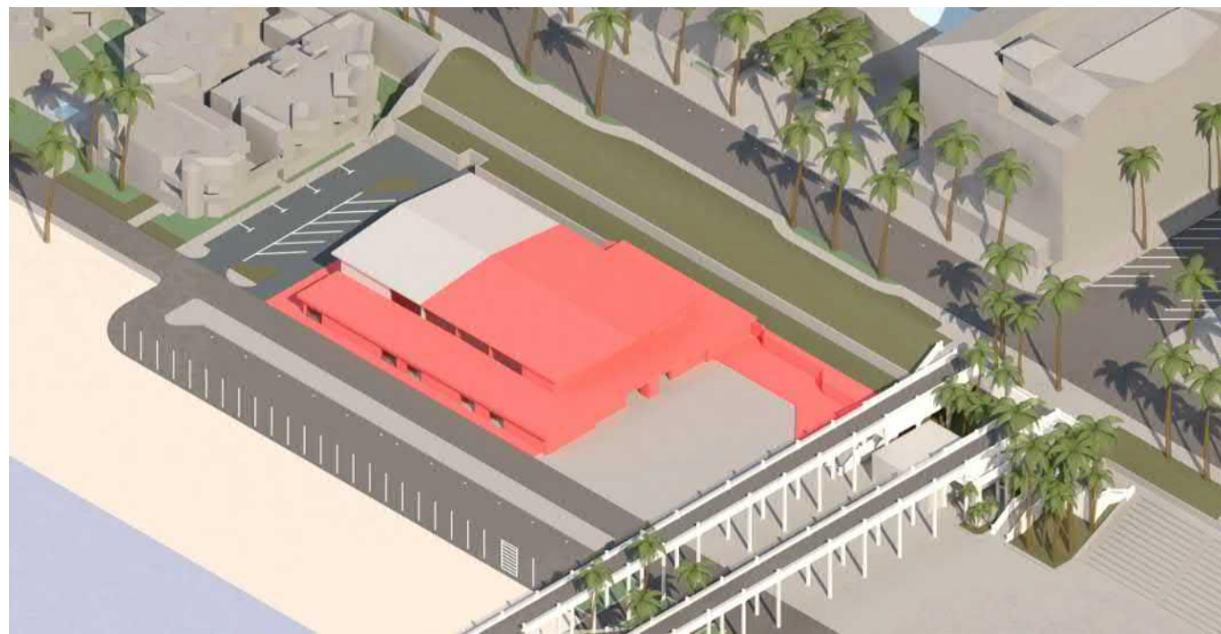
ADDITION AND RENOVATION More than half of the southern end of the building must be demolished in order to construct a regulation high school three court basketball court. The new court is both taller and wider than the current building structure allows.
