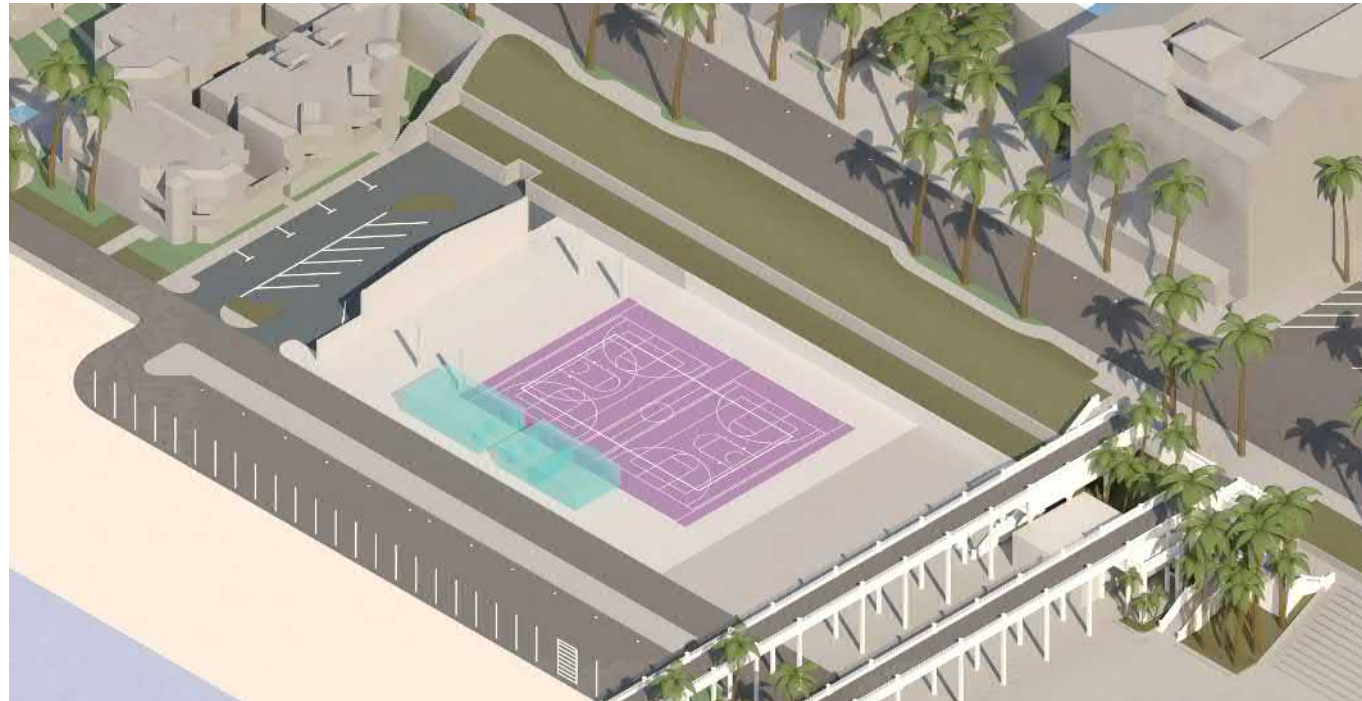
CLASSROOMS With construction of a new regulation court for both volleyball and basketball, existing classrooms that face the Strand are demolished (shown in blue). The classrooms are too narrow and too small and the new court area overlaps with required interior circulation access to the classrooms.
