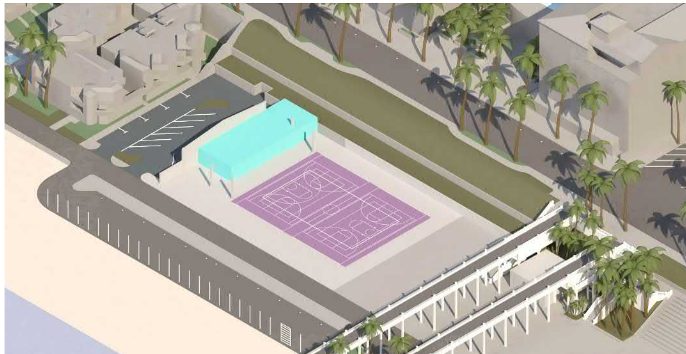
CLASSROOMS Two new larger and better proportioned recreation classrooms with storage (shown in blue) are built in the location of the existing stage.
