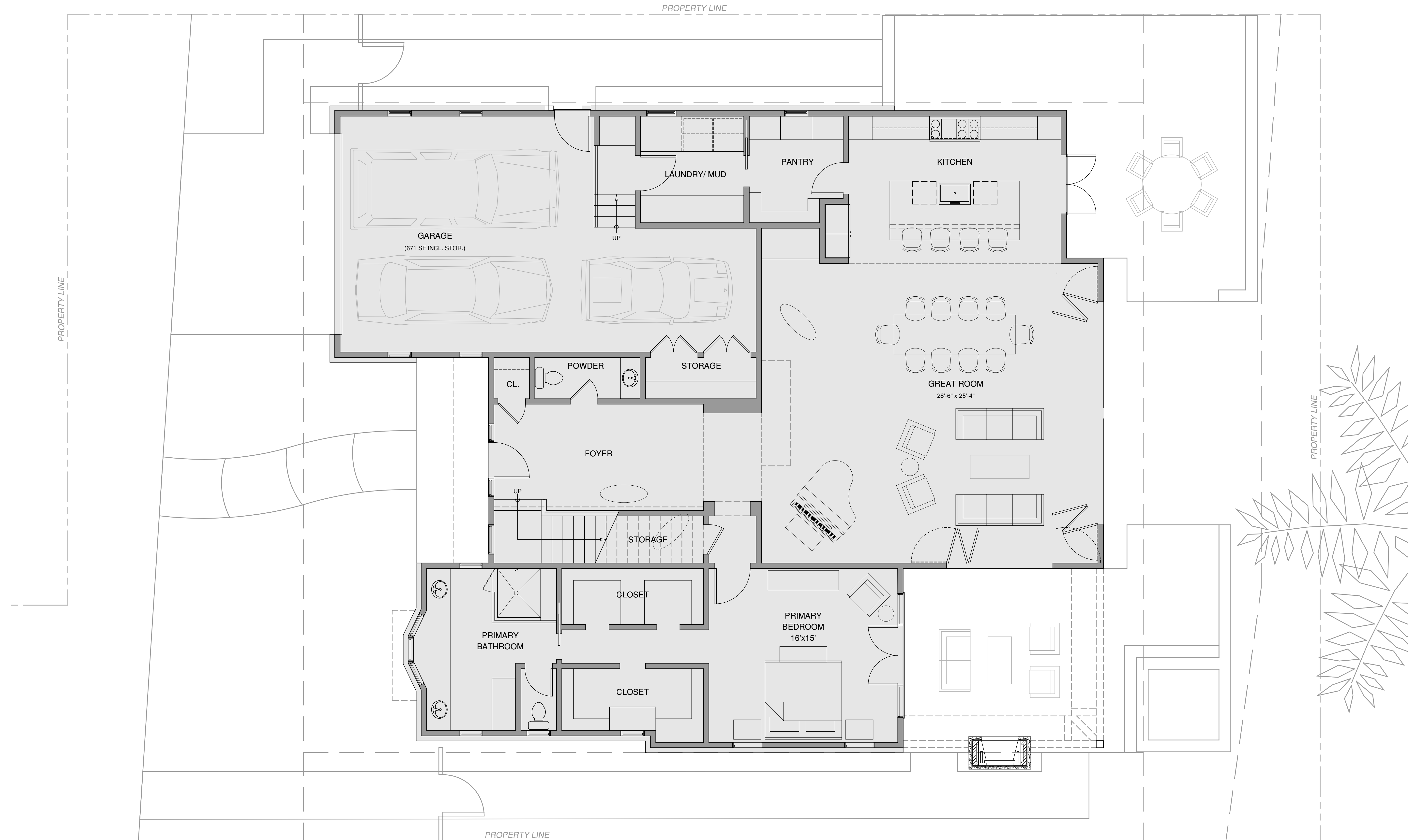
LOWER FLOOR PLAN - Scheme 2 (2,192 sf Living + 671 sf Garage = 2,863 sf) (2,807 sf Approved) Scale: 1/4"=1'-0"
